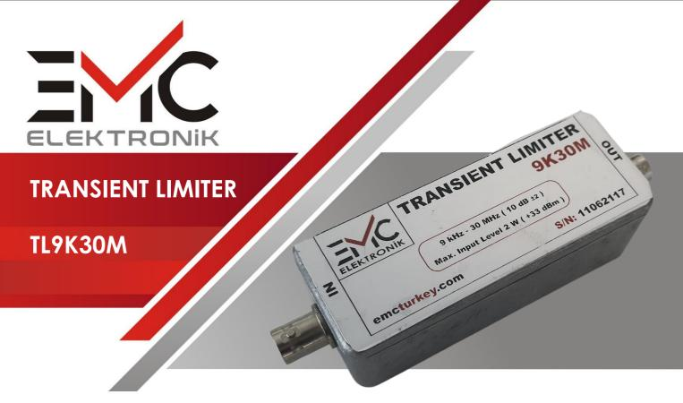
Transient Limiter, is used to protect RF input of the measuring receiver against high-level transients caused by LISN in conducted emission measurements. In addition, it has a high pass filter that prevents the effects of low frequency signals on the measuring receiver. Connector type and insertion loss is changeable upon request.
