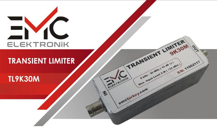
Transient Limiter, is used to protect RF input of the measuring receiver against high-level transients caused by LISN in conducted emission measurements. In addition, it has a high pass filter that prevents the effects of low frequency signals on the measuring receiver. Connector type and insertion loss is changeable upon request.
